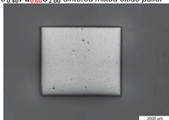
Optical microscopy observation of the obtained U_{0.40}Pu_{0.60}O_{2.00} sintered mixed oxide pellet
